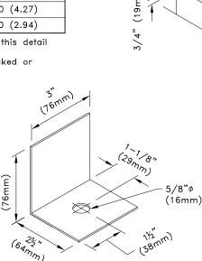
$\frac{\text{Clip A}}{\text{16 ga ASTM A653 SS Grade 33 G60}}$  Bare metal thickness, t = 0.0538" (1.37mm)
