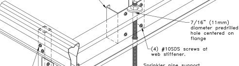
Sprinkler pipe support attached to rod.
