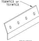
TS6WTC3 bare metal thickness (t) = 0.0538 in. (1.37mm) TS1WTC3
