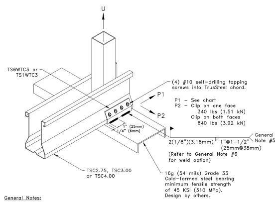
1. The wall top plate is to be designed by the job engineer. The wall top plate and connection of top plate to wall stud must be designed to support the loads applied to it (downward, upward
