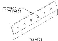
bare metal thickness (t) = 0.0538 in. (1.37mm) TS1WTC5
