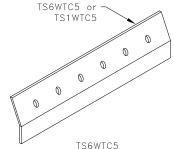
bare metal thickness (t) = 0.0538 in. (1.37mm) TS1WTC5
